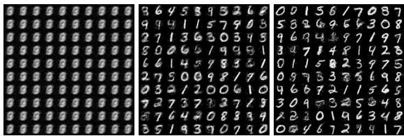
Figure 4. Prototypes learned using linear discriminator (left), dense discriminator (middle), and CNN discriminator (right).
